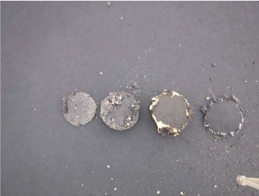
Non-Asbestos containing roof membrane (Bottom layer to the left, top to the right)
