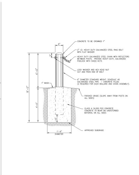
BOLLARD & CHAIN ASSEMBLY (STEEL PIPE) 53
