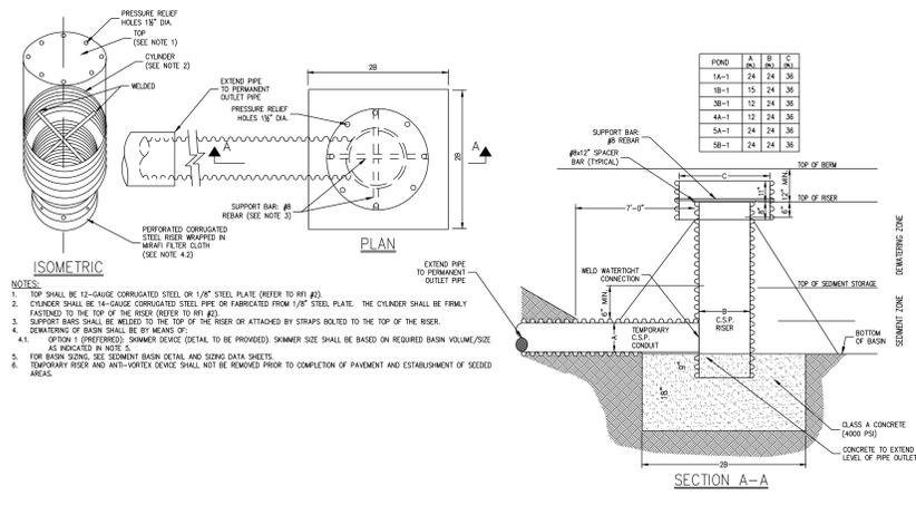
TEMPORARY RISER & ANTI-VORTEX DEVICE (FOR SEDIMENT BASIN) 81
