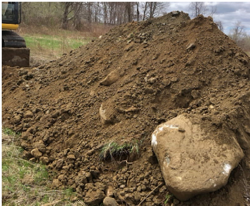
Photo 2: Excavated material from test pit LTP-14
