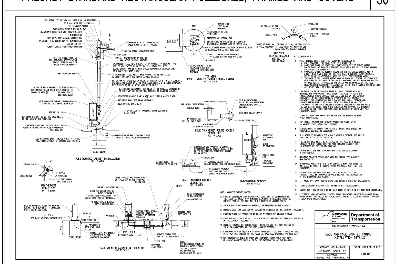
BASE AND POLE MOUNTED CABINET INSTALLATION DETAILS
