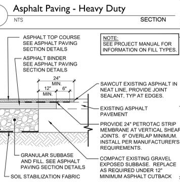
**4 Asphalt Paving at Existing Asphalt**
