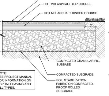
**3 Asphalt Paving - Heavy Duty**
