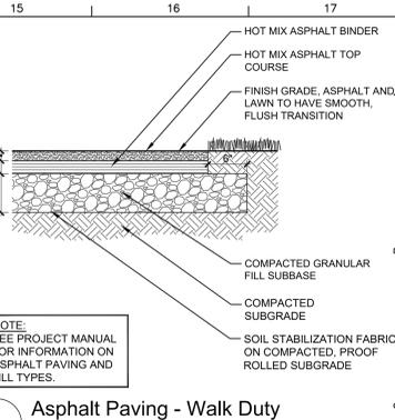
**1 Asphalt Paving - Walk Duty**
