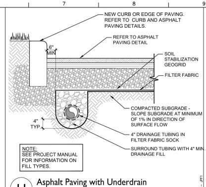
**11 Asphalt Paving with Underdrain**
