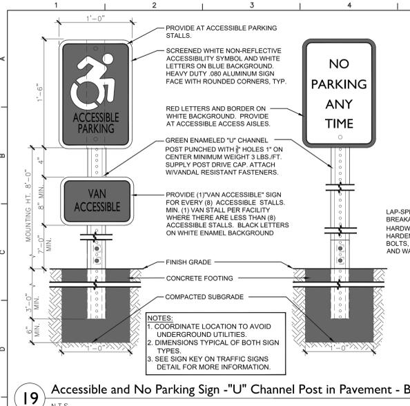
**19 Accessible and No Parking Sign - "U" Channel Post in Pavement - Breakaway Mount**
