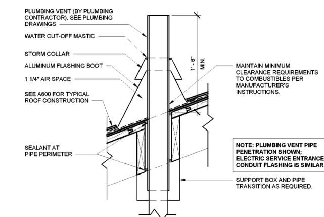
3 TYP. PIPE PENETRATION FLASHING DETAIL
