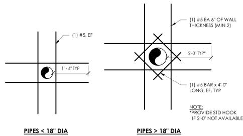
**6 TYPICAL PIPE OPENING IN CONCRETE WALL**
