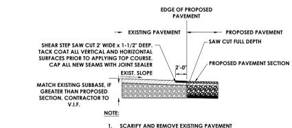
**13 PAVEMENT KEY DETAIL - CONNECTION TO (E) ASPHALT**
