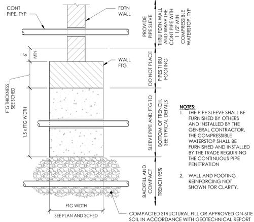
**1 TYPICAL PIPES AT FOUNDATION**
