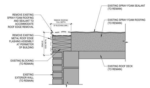
**2** ROOF EDGE FLASHING DEMOLITION
