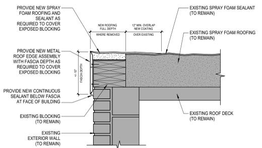
**3** NEW ROOF EDGE FLASHING
