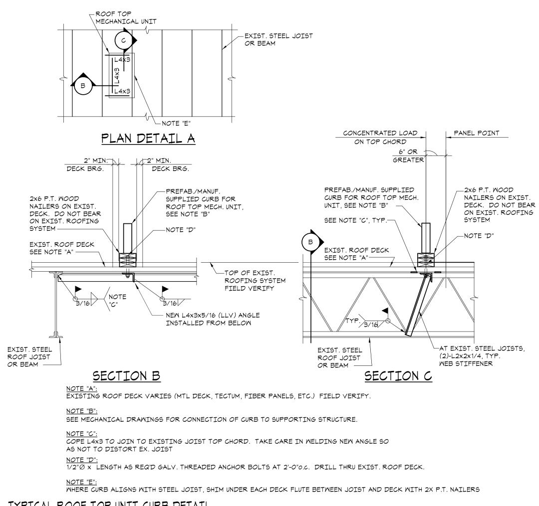
2 TYPICAL ROOF TOP UNIT CURB DETAIL
