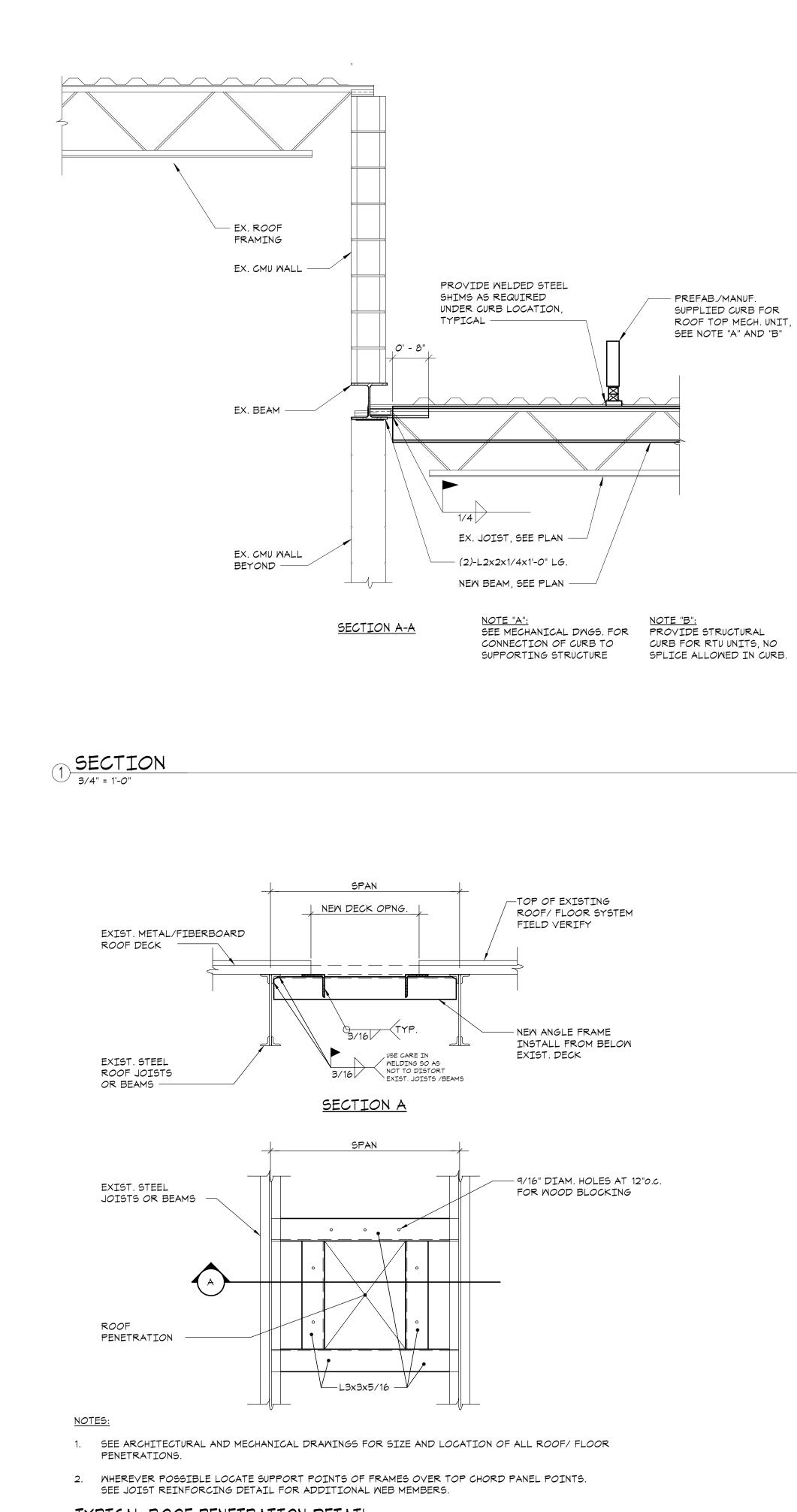
3 TYPICAL ROOF PENETRATION DETAIL
