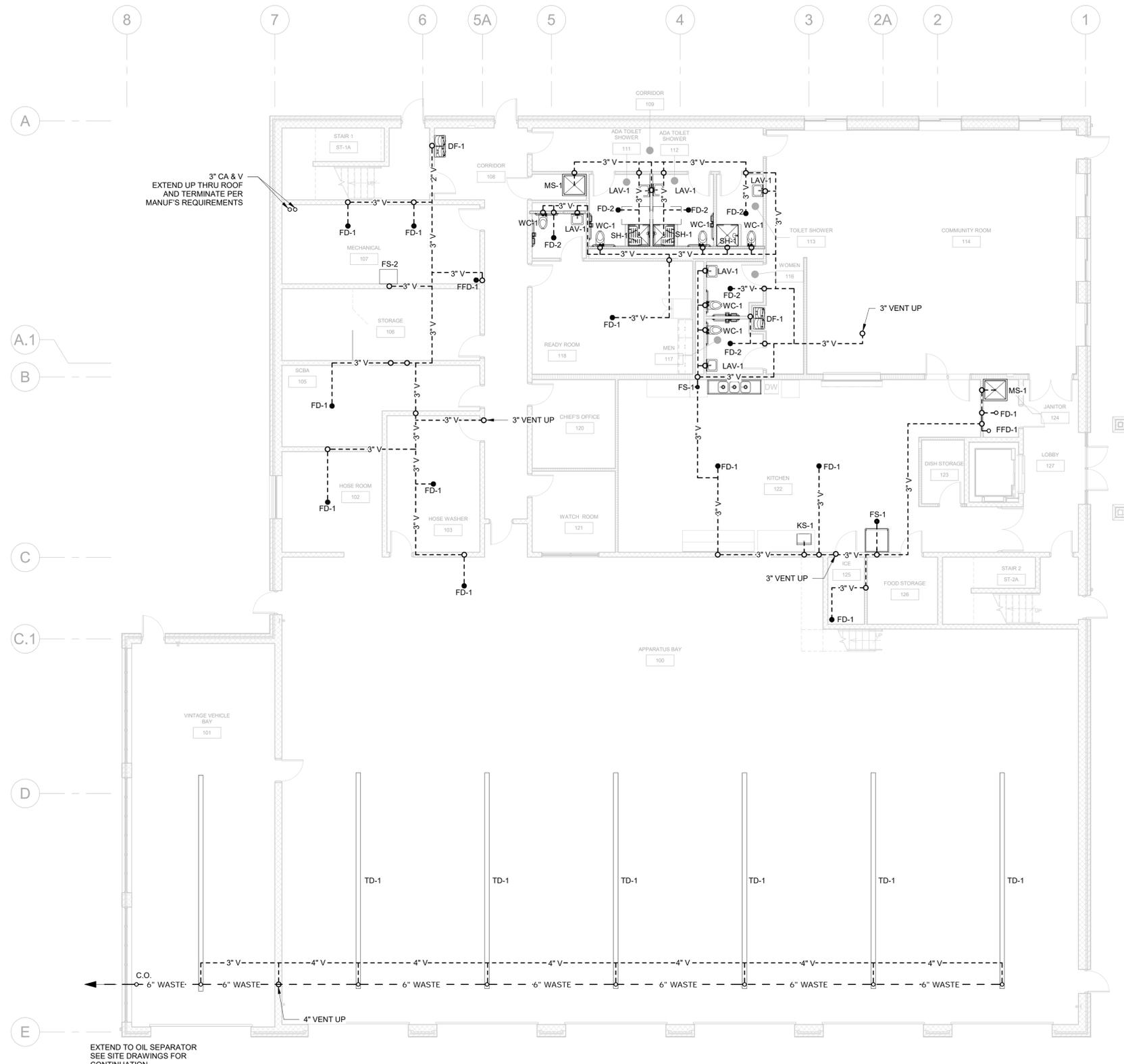
1 VENTING - FIRST FLOOR PLAN
