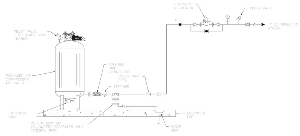
TYPICAL AIR COMPRESSOR INSTALLATION
