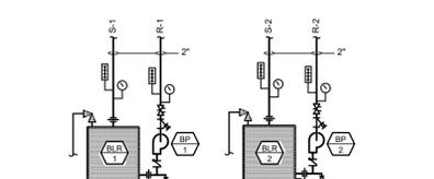
CONDENSATE TRAP. INSTALL CONDENSATE PIPE/TUBING IN ACCORDANCE WITH MANUF'S INSTRUCTIONS. (TYP.)
