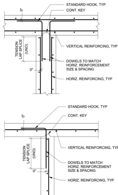
8 TYP CONCRETE WALL INTERSECTION DETAIL
