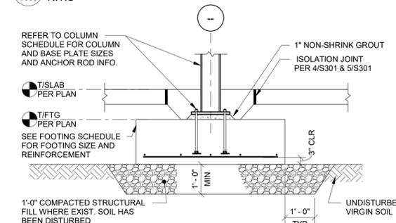
4 TYPICAL INTERIOR SPREAD FOOTING DETAIL
