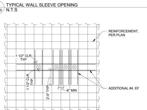
13 TYPICAL MULTIPLE WALL SLEEVE OPENING DETAIL
