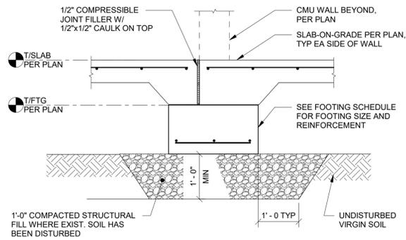
15 FOOTING AT INTERIOR MASONRY WALL OPENING
