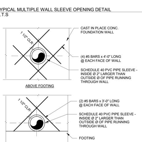
12 TYPICAL WALL REINFORCING FOR PIPE OPENING
