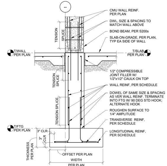
3 TYPICAL INTERIOR FOUNDATION WALL DETAIL - ALTERNATE 1
