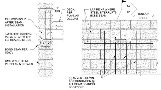
9 TYPICAL BEAM BEARING DETAIL @ NEW WALL
