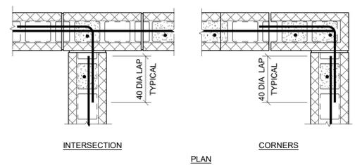
7 TYPICAL STRUCTURAL BOND BEAM IN CMU WALLS
