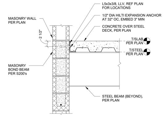
11 PERIMETER ANGLE AT MASONRY WALL
