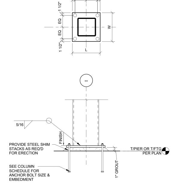
2 TYP COLUMN BASE DETAIL - TYPE 1 S700 N.T.S
