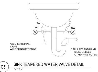
**C5** SINK TEMPERED WATER VALVE DETAIL
