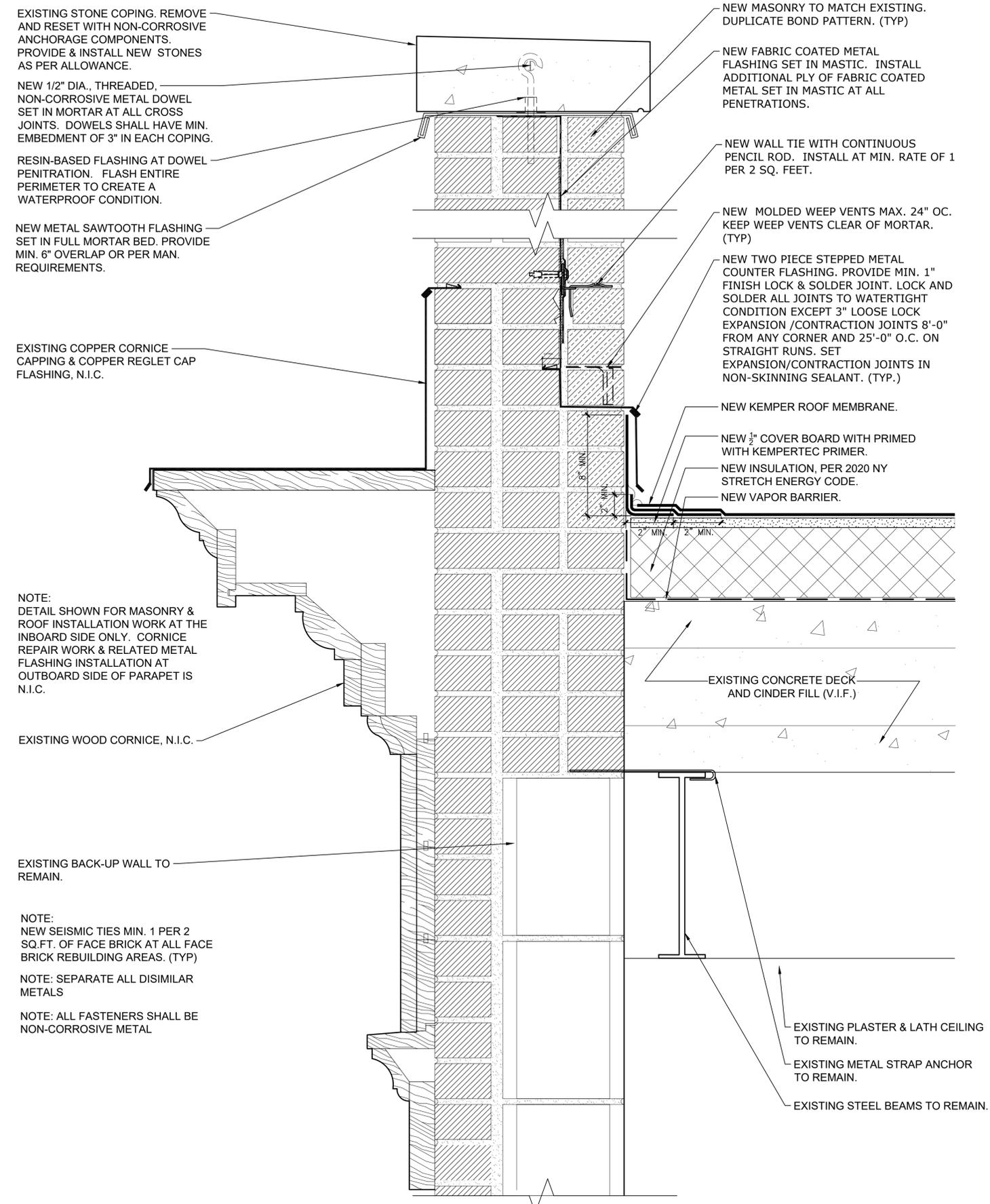
EXISTING STONE COPING. REMOVE AND RESET WITH NON-CORROSIVE ANCHORAGE COMPONENTS. PROVIDE & INSTALL NEW STONES AS PER ALLOWANCE.
