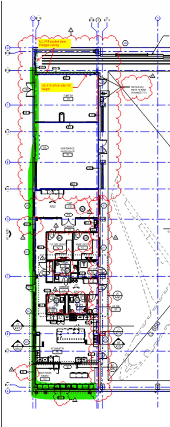
1. All exterior walls at conditioned office/shops spaces to have R-6.5 continuous rigid insulation attached to thermally broken z clips, and additional R-20 batt insulation within framing studs.
