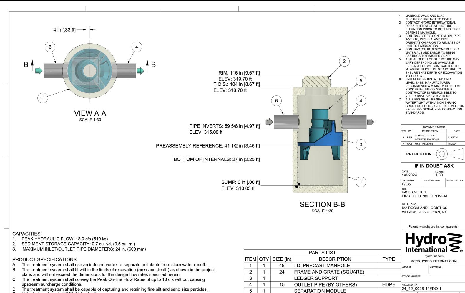
E. Unit shall conform to HS20-44 load ratings.
