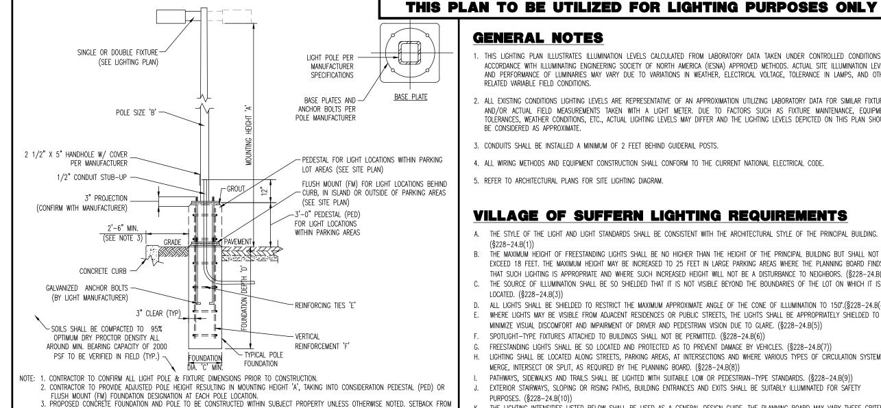
CURB IS PREFERRED BUT TO BE ADJUSTED AS NEEDED TO PREVENT ENCROACHMENT OVER PROPERTY LINE. 4. BASE PLATE & ANCHOR BOLTS PER POLE MANUFACTURER. LARGER FOOTING DIAMETER AND/OR ALTERNATE ARRANGEMENT OF REINFORCING TEEL MAY BE REQUIRED TO ACCOMMODATE ANCHOR BOLT CONFIGURATION. CONTRACTOR RESPONSIBLE TO COORDINATE DIMENSIONAL REQUIREMENTS FOR BASE PLATE, ANCHOR BOLTS & REINFORCING STEEL PRIOR TO CONSTRUCTION.
