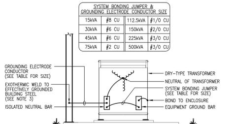
**TRANSFORMER GROUNDING SCHEMATIC**
