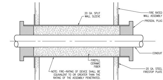
**CONDUIT THROUGH FIRE RATED WALL**
