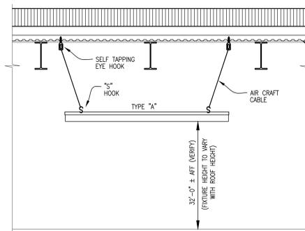
**FIXTURE TYPE "A" MOUNTING DETAIL**
