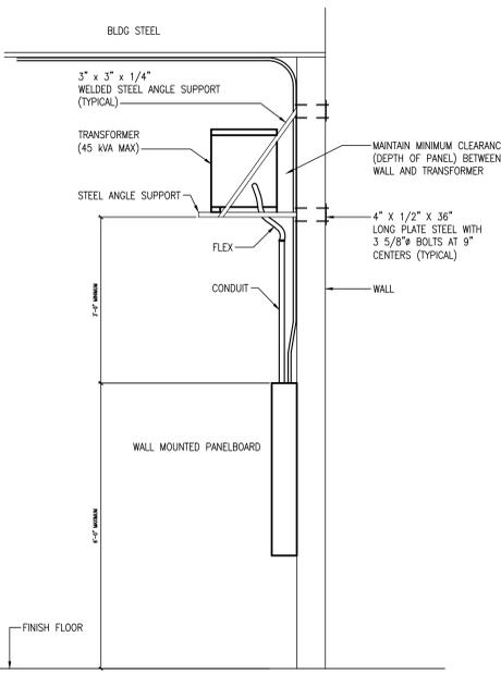
**TRANSFORMER WALL MOUNTING DETAIL**
