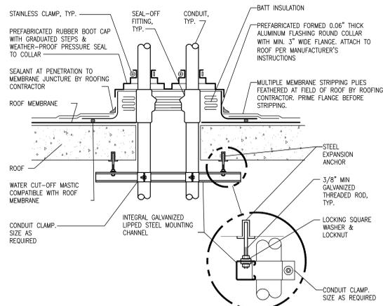
**TYPICAL ROOF PENETRATION DETAIL**
