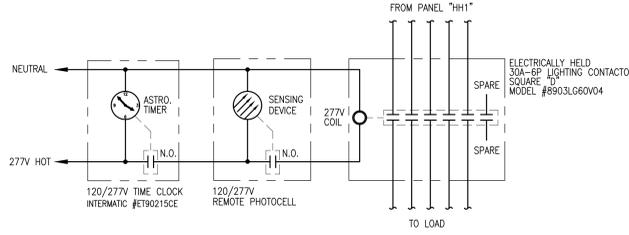
**TIMECLOCK/PHOTOCELL SCHEMATIC DIAGRAM**
