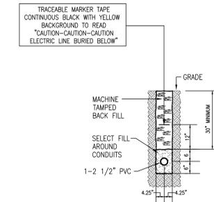
**SECTION "C-C" DUCT BANK DETAIL**
