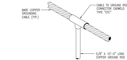
**CONTINUOUS CABLE TO GROUND ROD CONNECTION**
