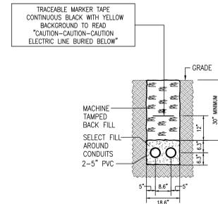
**SECTION "A-A" PRIMARY DUCT BANK DETAIL**
