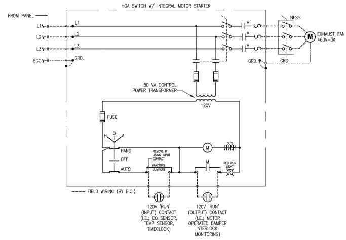
**TYPICAL 3-PHASE EXHAUST FAN CONTROL SCHEMATIC**
