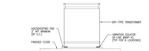
**TRANSFORMER FLOOR MOUNTING DETAIL**
