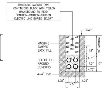
**SECTION "B-B" DUCT BANK DETAIL**
