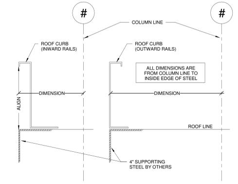
1 HVAC - ROOF CURB - DIMENSIONING DETAIL NTS
