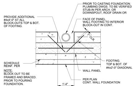
**FOOTING BLOCKOUT AT DOWNSPOUT, ROOF DRAIN, AND UTILITY**
