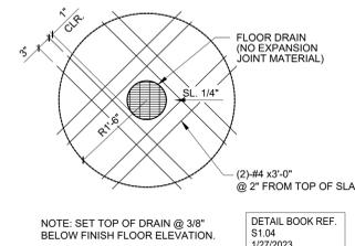
**FLOOR DRAIN PLAN DETAIL**
