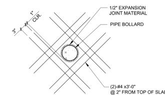
**REBAR @ PIPE BOLLARDS**
