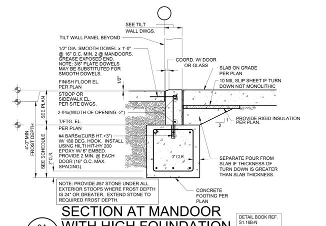
**SECTION AT MANDOOR WITH HIGH FOUNDATION & INSULATION**
