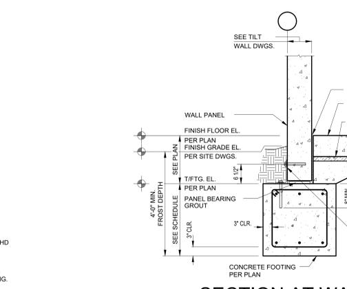
**SECTION AT WALL WITH HIGH FOUNDATION & INSULATION**
