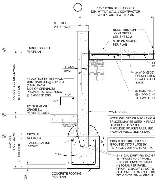
**WALL FOOTING AT TILT WALL PANEL AT DOCK WALL**
