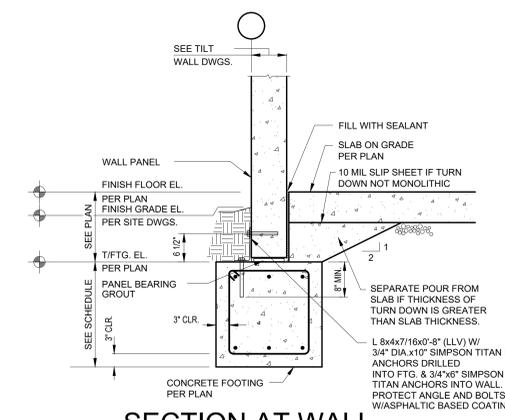
**SECTION AT WALL WITH HIGH FOUNDATION**
