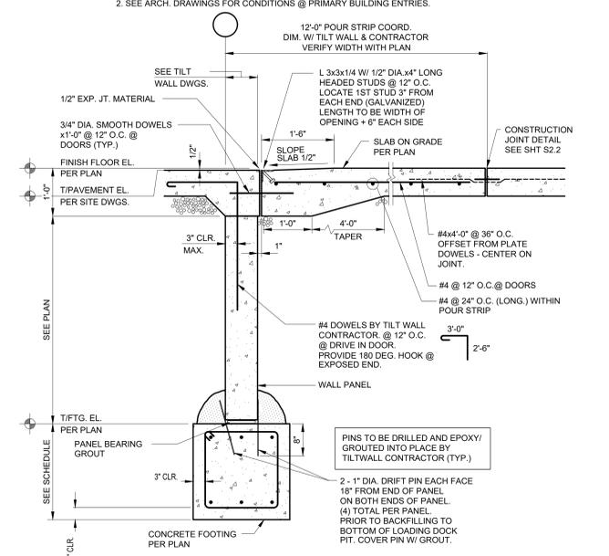
**SECTION AT DRIVE-IN DOOR WITH LOW FOUNDATION**
