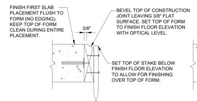
**PLATE DOWEL CONSTRUCTION JOINT INSTALLATION**
