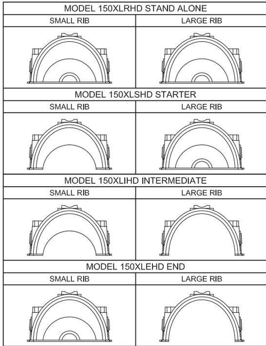
CULTEC RECHARGER 150XLHD CHAMBER STORAGE = 2.65 CF/FT [0.246 m<sup>3</sup>/m]
