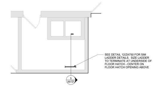
3 1st Floor - Area B - Partial Plan
