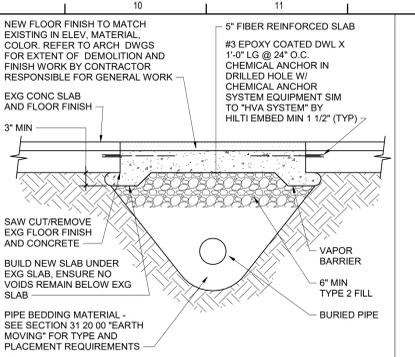
**4 Trenching Below Existing Slab Detail**
