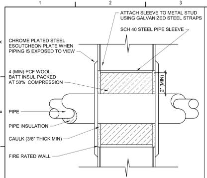
**7 Fire Rated Metal Stud Wall Sleeve Detail**
