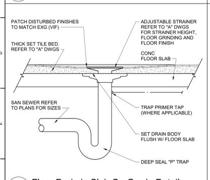
**11 Floor Drain in Slab On Grade Detail**
