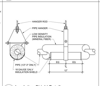
**9 Insulation Shield Detail**
