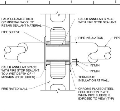
**6 Fire Rated CMU Wall Pipe Sleeve Detail**
