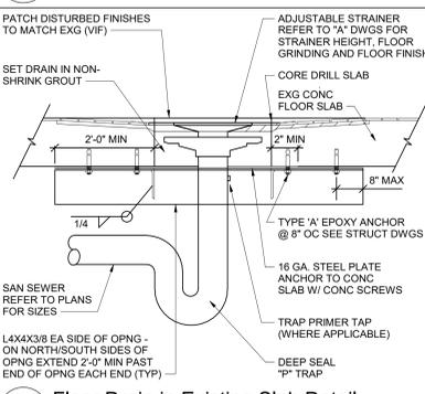
**10 Floor Drain in Existing Slab Detail**
