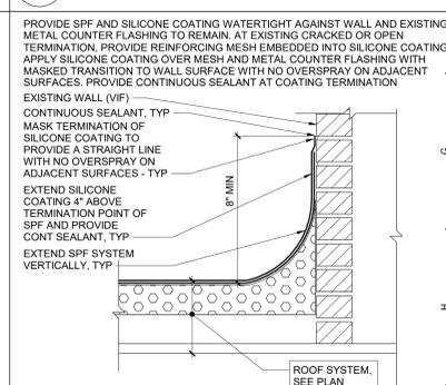
**3 SPF Base Flashing Detail at Wall**
