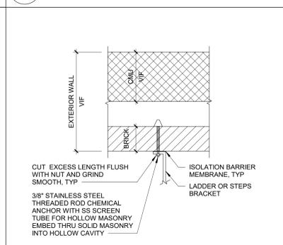
**7 Ladder Anchor Detail at Exterior**
