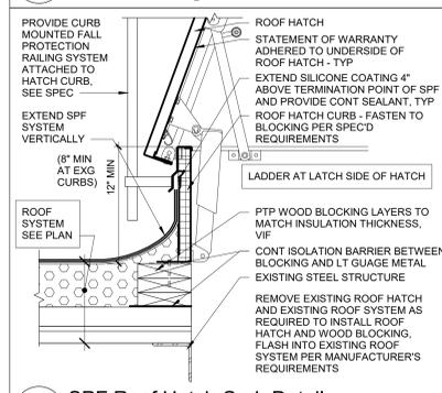
**11 SPF Roof Hatch Curb Detail**
