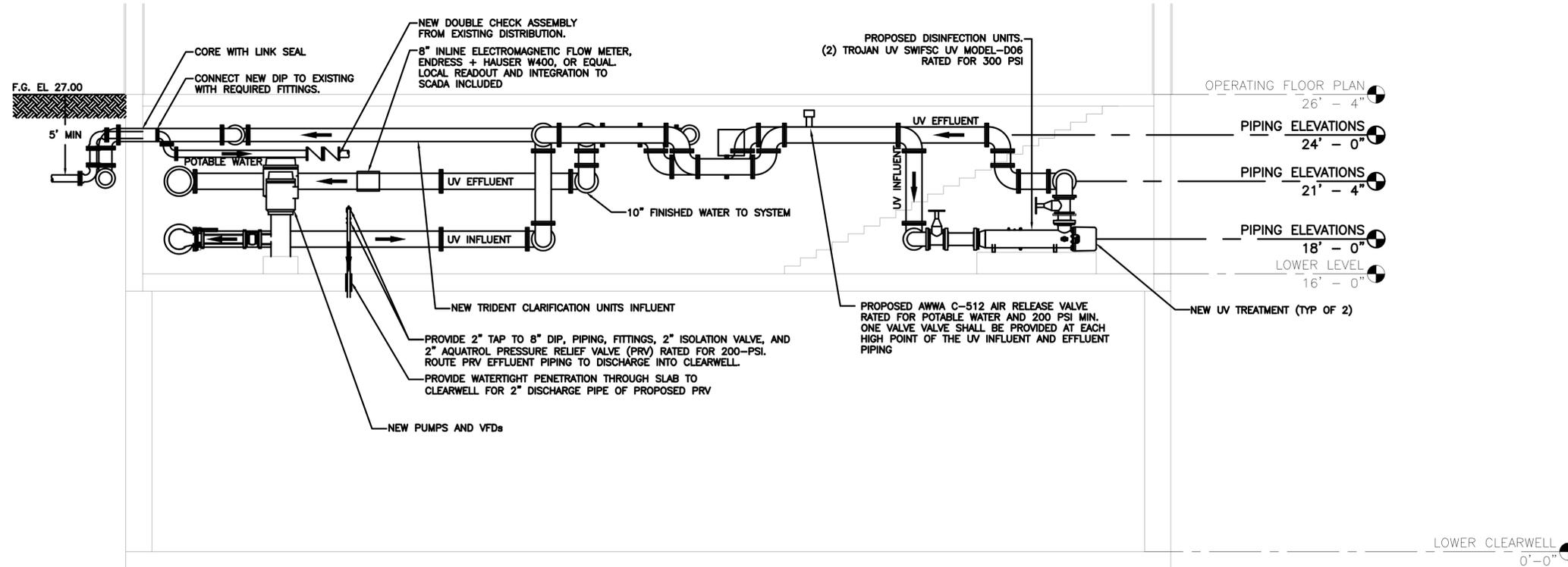
B FILTER AND UV TREATMENT PIPING SECTION
