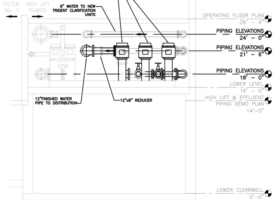
(3) NEW HIGHLIFT PUMPS, 700 GPM @ 422 TDH, GOULDS VT-12WAHC, OR EQUAL. PROVIDE ISOLATION VALVES, SWING CHECK VALVES WITH CLOSED LIMIT SWITCHES AND EXTERNAL SPRING-LOADED LEVERS, REQUIRED FITTINGS, PRESSURE GAUGES, AND CONTROLS
