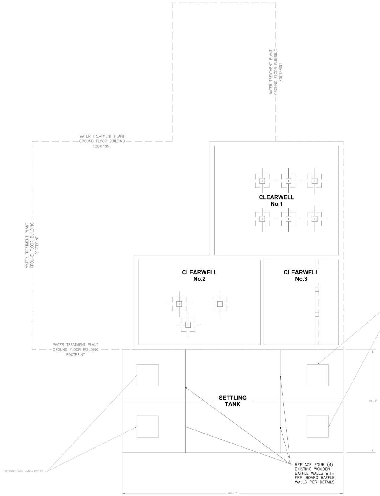
**PROPOSED UPGRADES TO EXISTING SETTLING TANKS**
