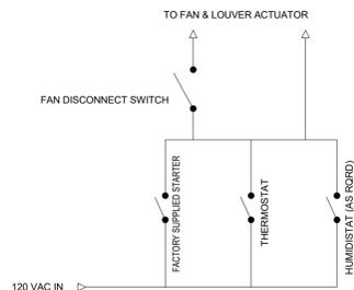
TYPICAL EXHAUST FAN WIRING SCHEMATIC
