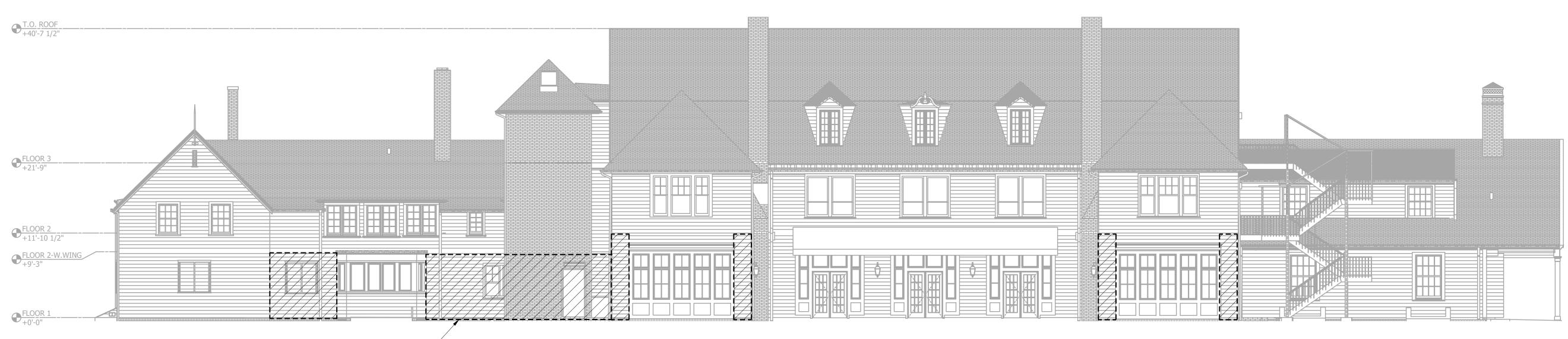
WHERE SHADED THUS, REMOVE FINISHES AND — SHEATHING TO EXPOSE VERTICAL WOOD BEARING STUDS FOR THEIR FULL FIRST STORY HEIGHT AND REPLACE NON-COMPLIANT PER A/S500
