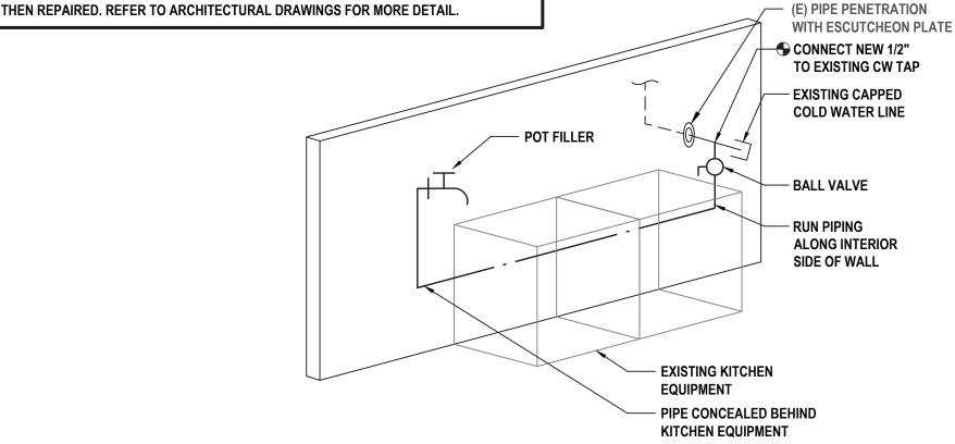
Pot Filler Plumbing Routing Detail
