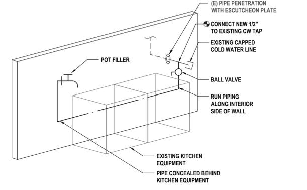
**3 Pot Filler Plumbing Routing Detail**
