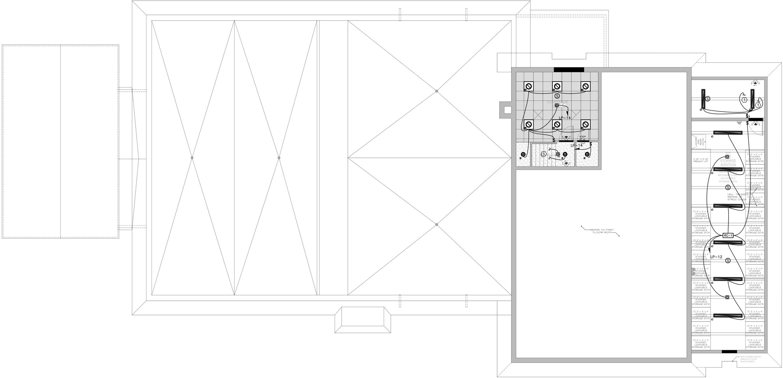
**1 ELECTRICAL: CONSTRUCTION SECOND FLOOR LIGHTING & FIRE ALARM PLAN**
