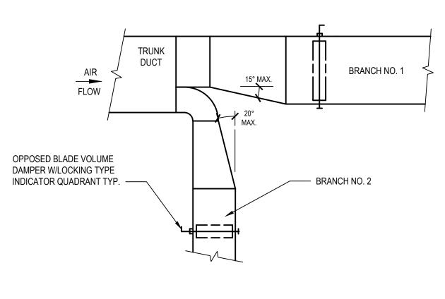
1. FURNISH THIS TYPE OF CONNECTION WHEN SINGLE LINE DUCTWORK IS INDICATED AS SHOWN FOR LOW PRESSURE BRANCHES WITH 33% OR MORE CAPACITY OF THE MAIN DUCT.
