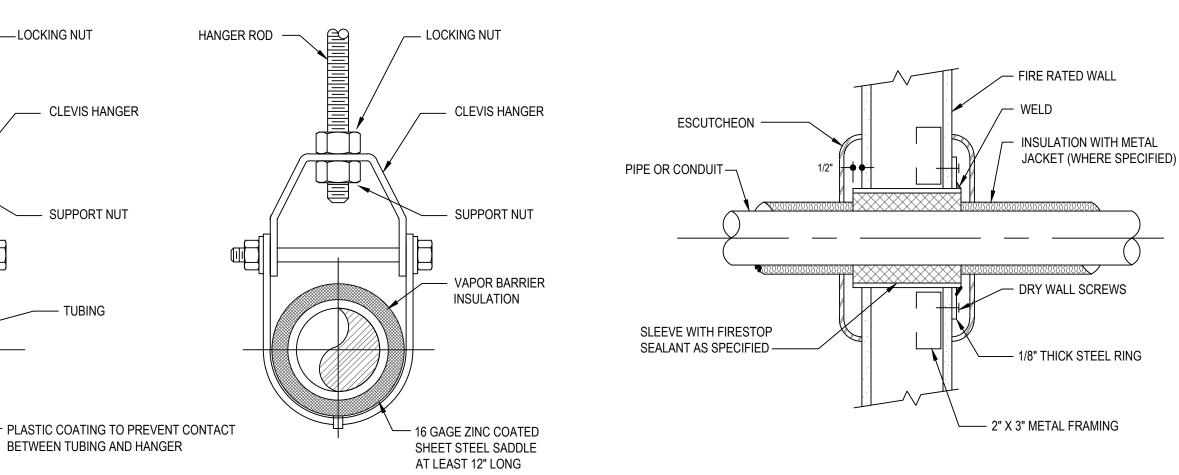
Pipe or Conduit Penetration Through Fire Rated Walls
