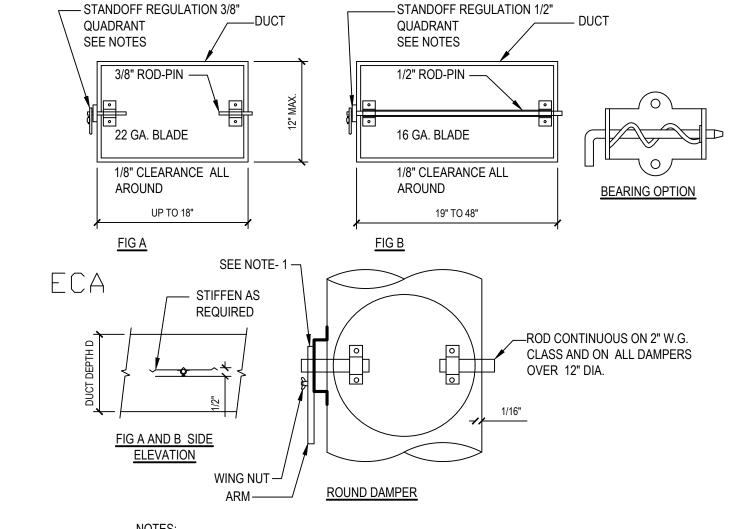
1. PROVIDE 2" HIGH STANDOFF REGULATORS FOR EXTERNALLY INSULATED DUCTWORK. PROVIDE REGULATORS WITH SEALS. DURO-DYNE MODEL E50.
