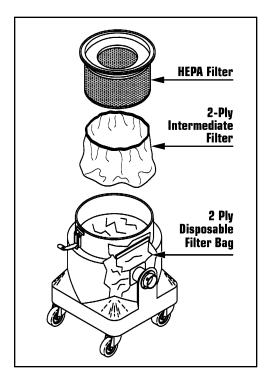
This hazardous waste vacuum has special filters installed. The 2-ply disposable paper bag filter contains the bulk of all debris and protects remaining filters from excess dirt. The 2-ply intermediate filter is a very fine non-woven filter that extends the life of the expensive High-Efficiency Particulate Air (HEPA) filter.
