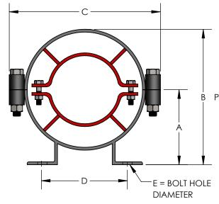
SPIDER SPACERS CENTER PIPE IN HOUSING AND ARE SIZED TO ALLOW INSULATION TO BE PACKED AROUND PIPE SPLIT HOUSING FOR EASY INSTALLATION MVMT . FEET CAN BE **BOLTED OR** WELDED TO **DIRECTION OF STRUCTURE** PIPE MOVEMENT \*EXTENDED SPIDER GUIDES ARE AVAILABLE. CONTACT METRAFLEX FOR OPTIONS. LEADING EDGE OF
