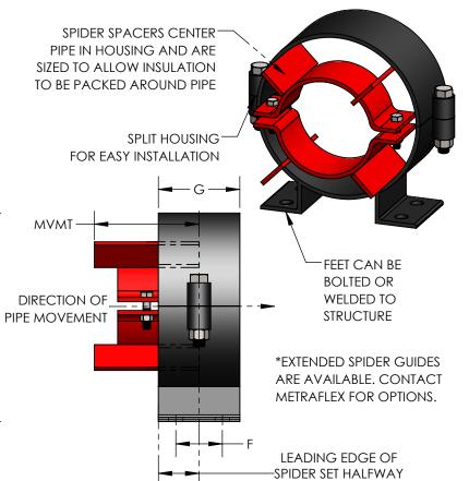
PROVIDES LATERAL STABILITY TO THE PIPE TO PREVENT "BOWING".
