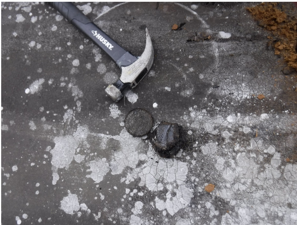
Original Building Roof (Roof over Lounge): Asbestos containing built-up layer.
