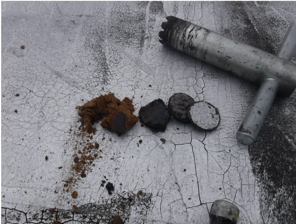
New Building Exterior Roof: Non-asbestos containing silver top layer, black 2 nd layer, fiberboard, and tar patches. Asbestos containing built-up layer.
