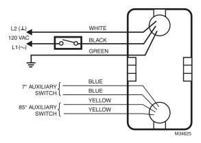
Fig. 4. Typical 120 Vac wiring.
