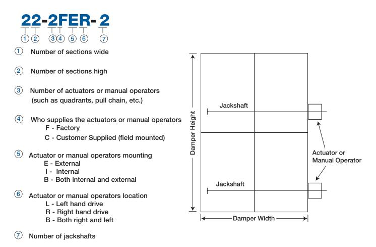
Each damper is supplied with a Drive Arrangement Prefix to help describe its construction. See the following examples:
