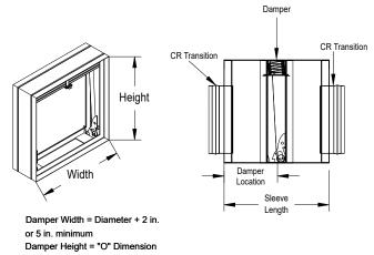
• This drawing shows a general damper configuration and is not intended to depict the exact configuration of all dampers in this submittal.
