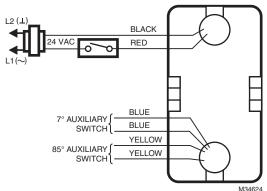
Fig. 3. Typical 24 Vac wiring.
