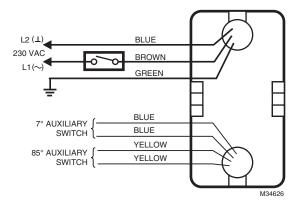
Fig. 5. Typical 230 Vac wiring.
