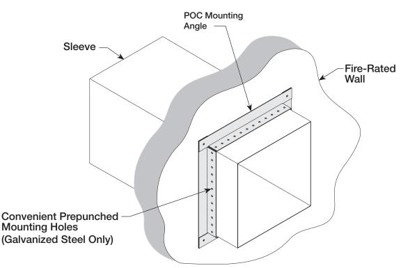
Retaining angle as mounted in the field.
