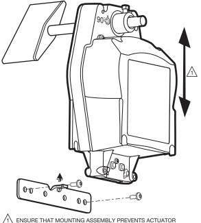
(1) ENSURE THAT MOUNTING ASSEMBLY PREVENTS ACTUATOR ROTATION AND ALLOWS ACTUATOR TO FLOAT ALONG INDICATED AXIS. WHEN TOO TIGHT, THE RESULTING BINDING CAN DAMAGE THE ACTUATOR OR REDUCE TORQUE OUTPUT. M34623A M34623A
